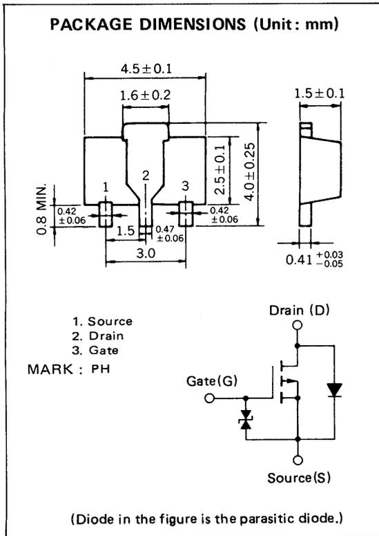
The 2SJ206, P-channel vertical type MOS FET, is a switching device which can be driven directly by the output of ICs having a 5 V power source.
